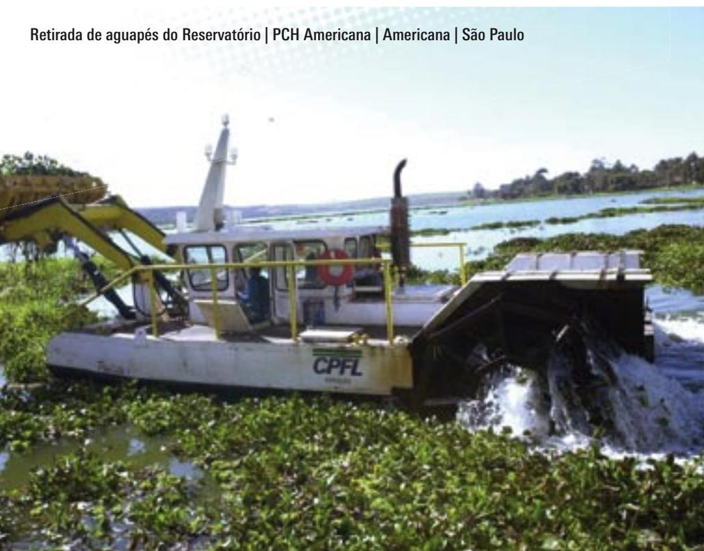
**3. Aquatic Plant Monitoring Program** – 2006 saw the practical implementation of a project first developed through R&D studies for the collection and mechanical shredding of aquatic plants found in CPFL plant reservoirs. A total of 38,017m<sup>3</sup> of this material was removed (equivalent to 60.30 ha). Studies are being developed to find the best end use for this type of aquatic plant.
